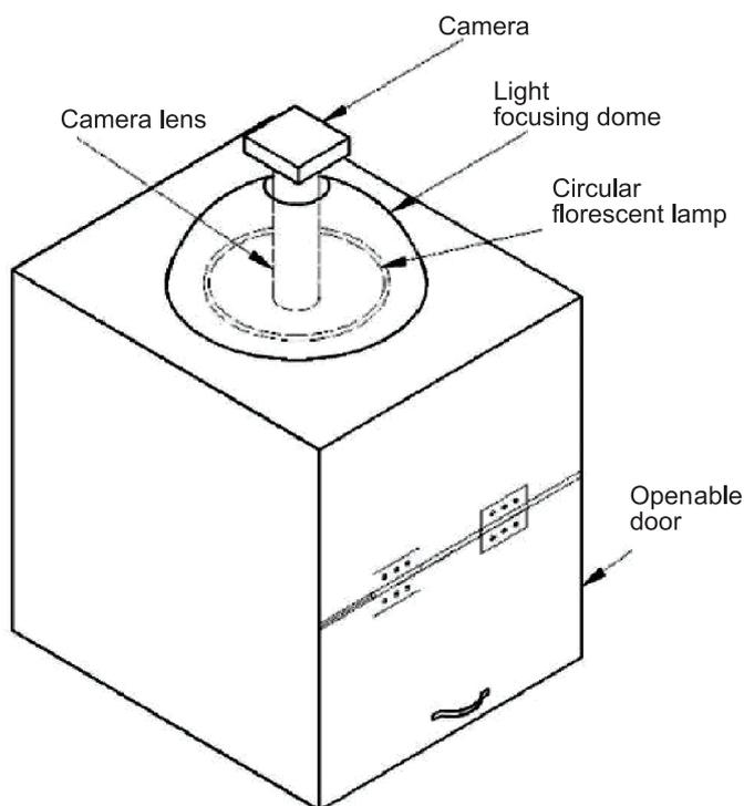
Fig. 1. Schematic diagram of image capturing setup
